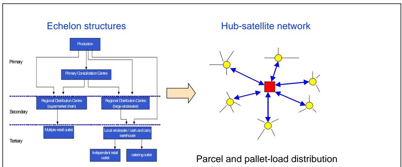
**Figure 4: Shift from Echelon to Hub-Satellite Networks**
